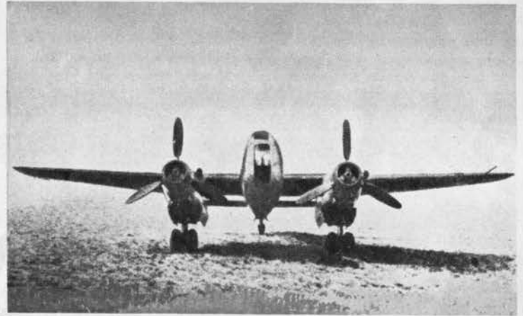
Low midwing with underslung nacelles marks Ar-240 when seen head-on. Cockpit set forward makes plane's nose look tall and thin.
